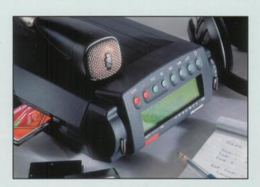
or stopped using the according buttons. During recording, headphone or speakervolume can be changed as well as recording level and gain, using the gain button.
